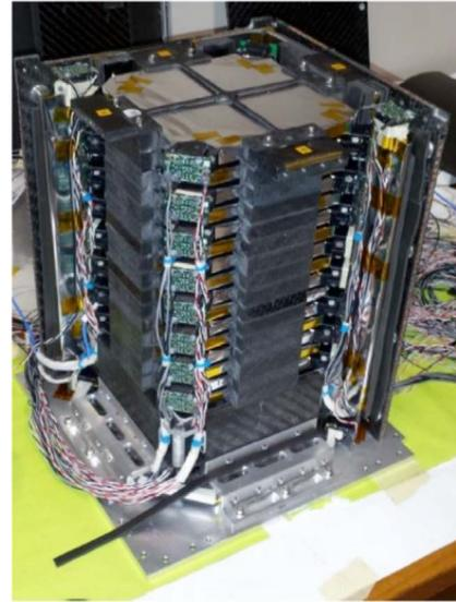
**Figure 18.** Picture of the assembled scintillator tower.
