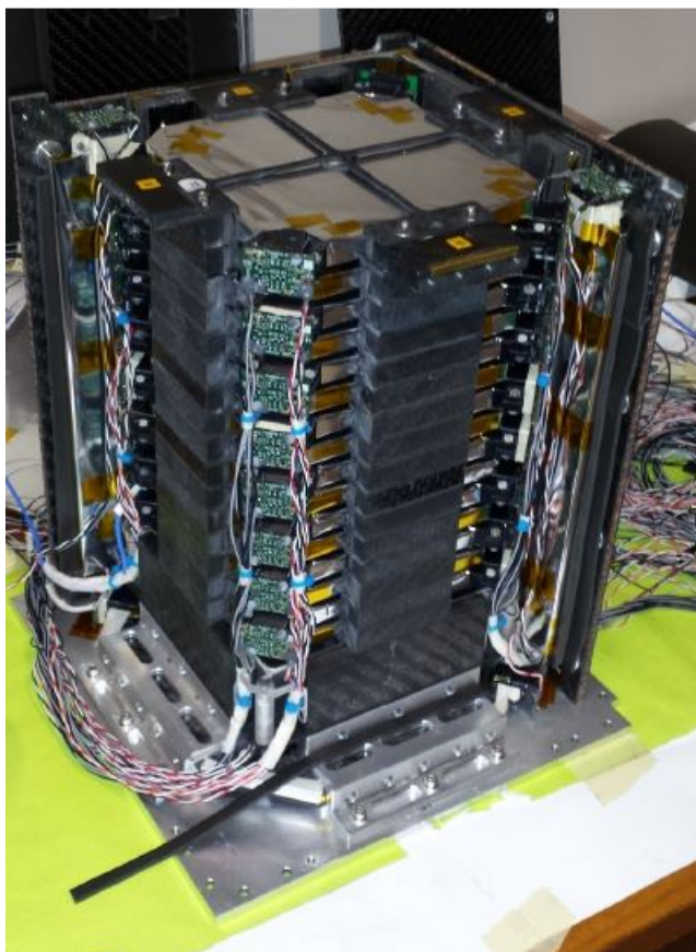
Figure 1.10: Calorimeter of HEPD-01 detector [15].
