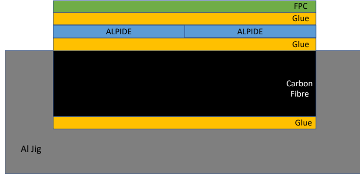
Figure 3.23: Stratigraphy of DUT. Different layers are not in scale.
