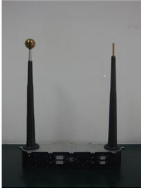
FIGURE 2.8: The two spherical Langmuir probes.
