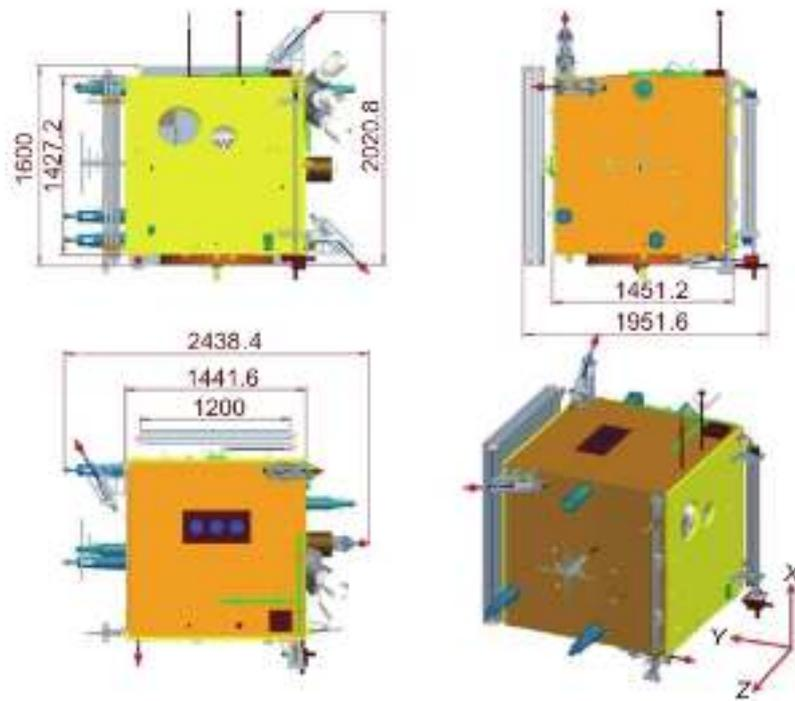
FIGURE 2.4: Several views of the CSES layout with the 4 telescopic booms of the EFD probes stowed. The search-coil magnetometer boom is folded at the edge between the XZ and the XY planes.
