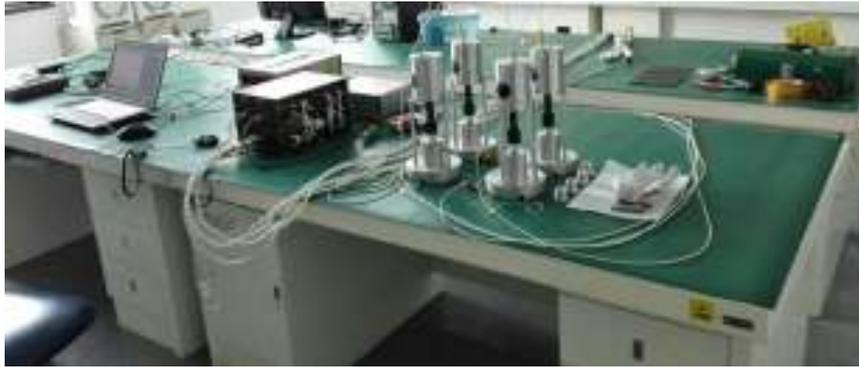
FIGURE 2.7: The four independent sensors composing EFD.
