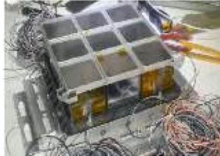
FIGURE 3.7: The matrix of  $3 \times 3$  LYSO blocks during integration.
