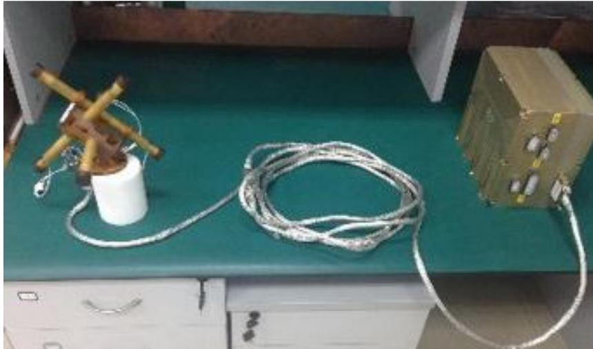
FIGURE 2.6: The search coil magnetometer.
