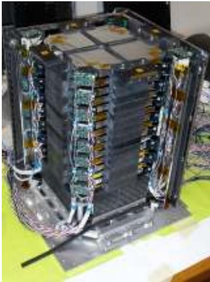
FIGURE 3.6: The tower of 16 planes during integration. The LYSO matrix, on the bottom of the instrument, is not visible.
